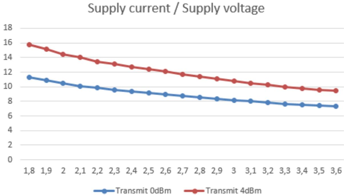
Figure 2: TX Current consumption vs. VCC
