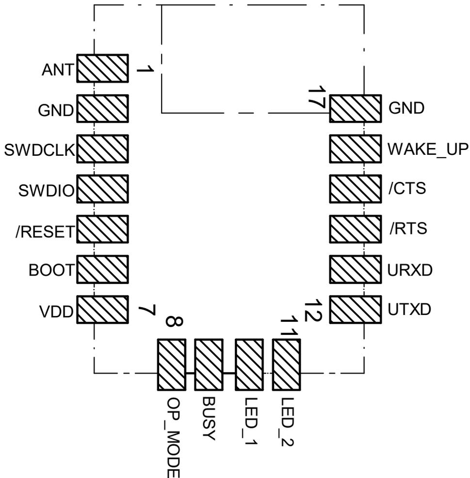
Figure 5: Pinout (top view)
