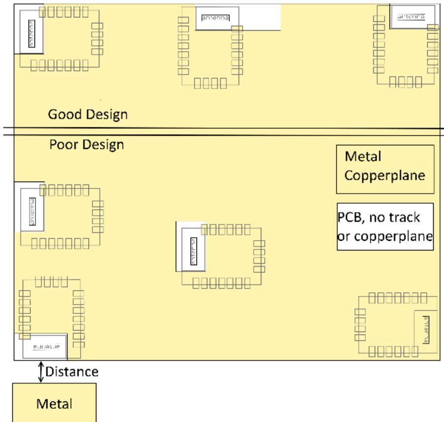
Figure 10: Placement of the module with integrated antenna
