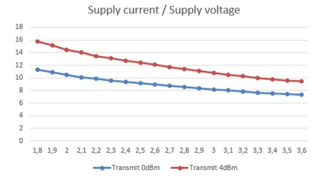
Figure 2: TX Current consumption vs. VCC
