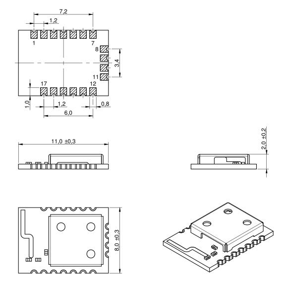
Figure 17: Module dimensions [mm]
