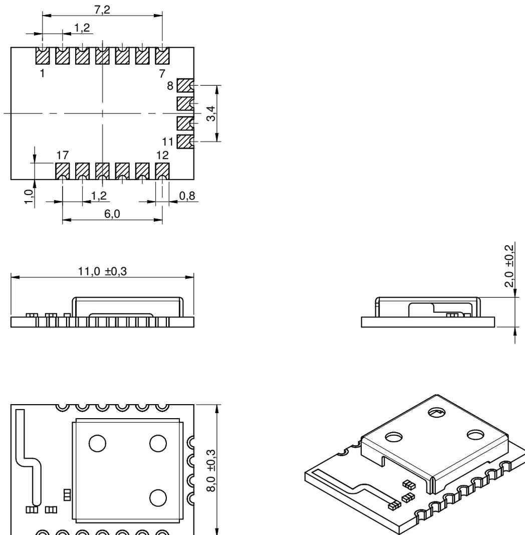
Figure 17: Module dimensions [mm]
