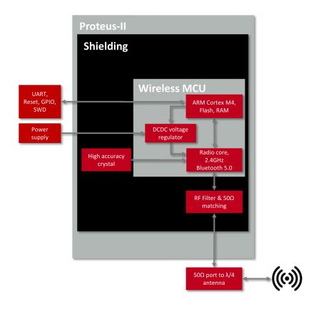
Figure 1: Block diagram of the module with internal PCB antenna and antenna pad
