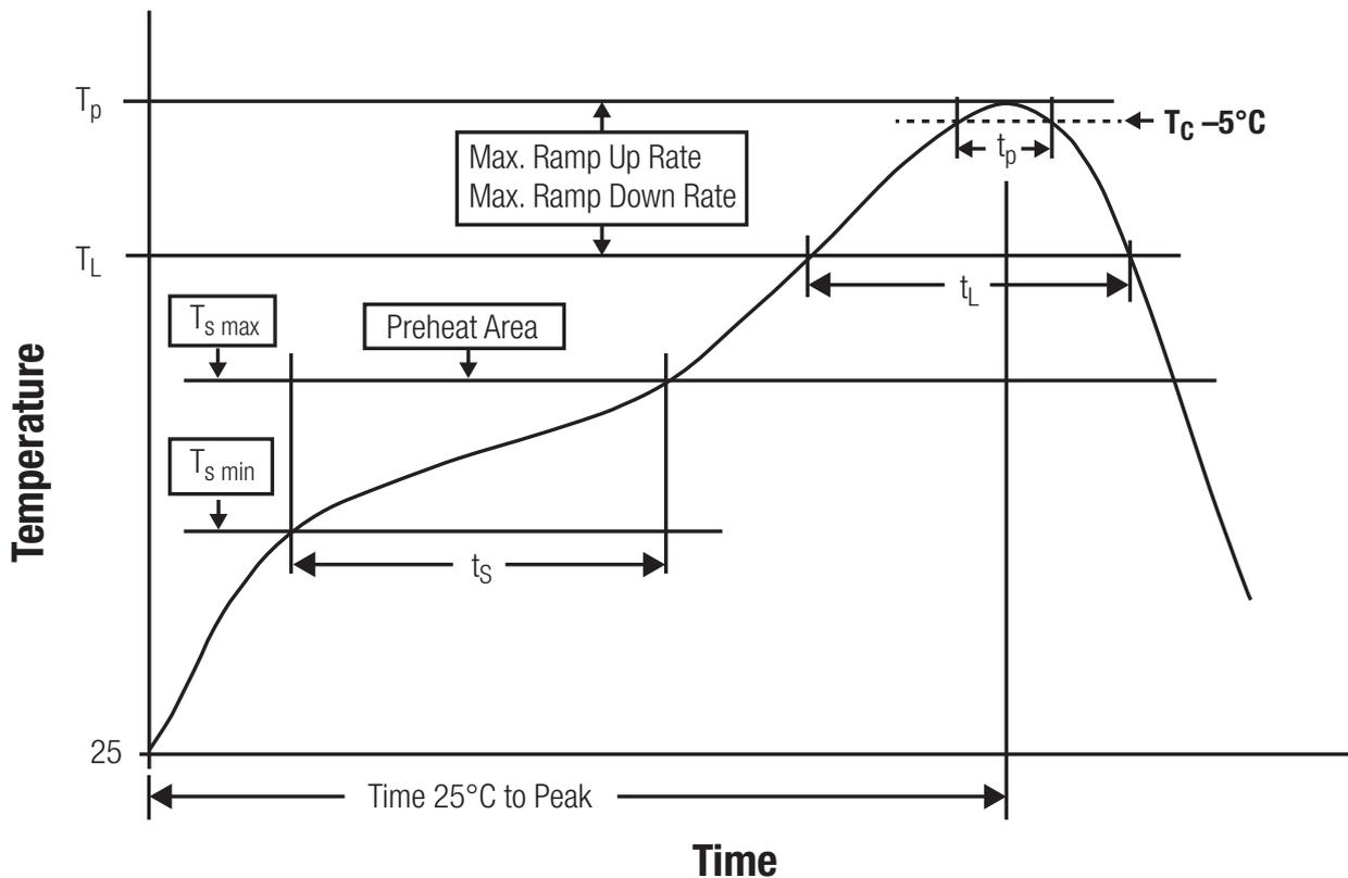
Figure 16: Reflow soldering profile
