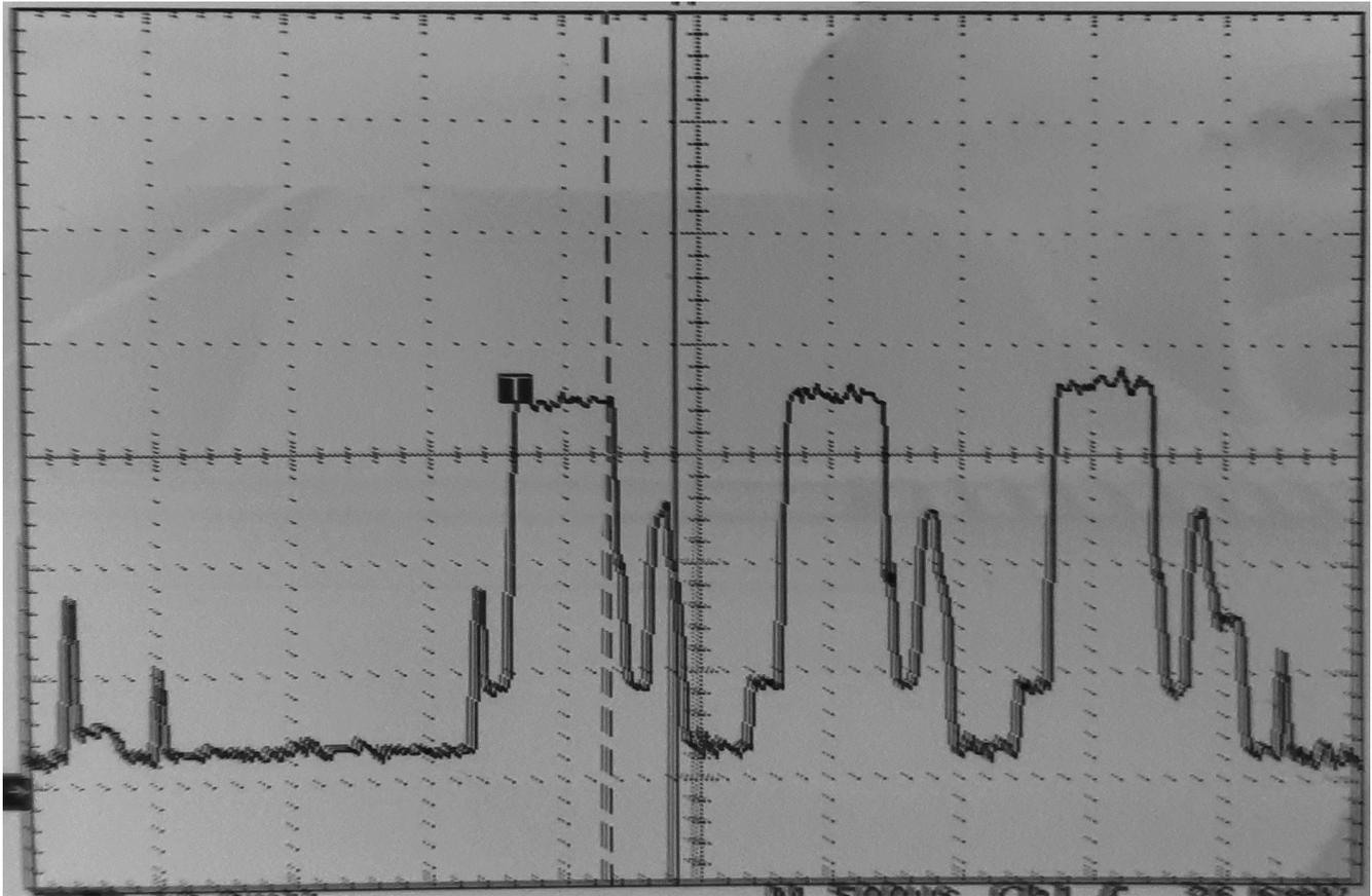
Figure 4: Measured Proteus-II transient current consumption in advertising mode with 40ms advertising interval, excerpt of 5ms
